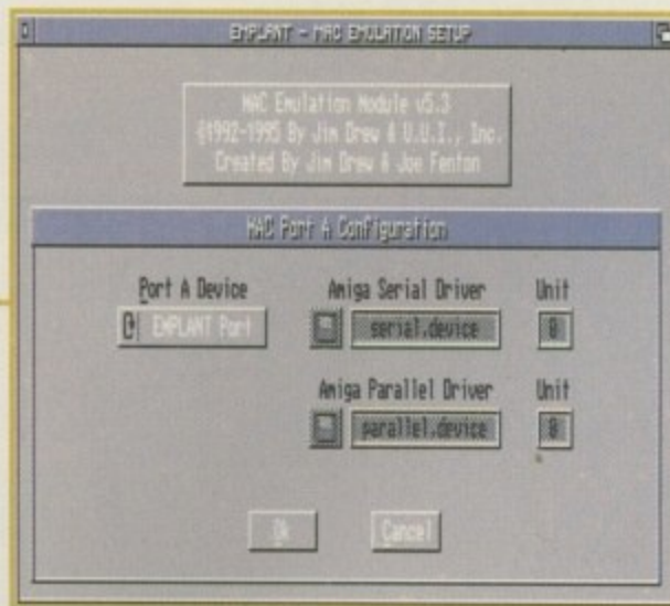
Both Mac emulators offer serial and parallel port emulation, but only Emplant actually has Mac serial ports
